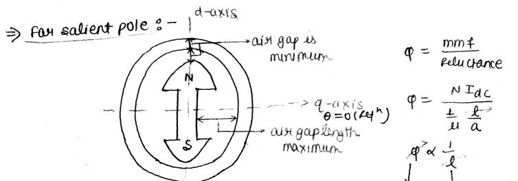
solby puofiling face of notay pole vory aix gap length So that flux will have cosine function.
