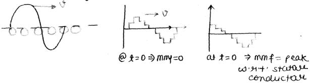
mmf wave : odd + Half wave symmetric Then, all sine tem with odd harmonic.
